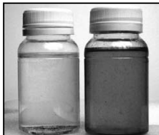
Contaminated private wells (sample at left) started showing up soon after firefighting efforts started, and worsened as time progressed (sample at right).
