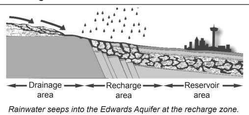
An aquifer is a geologic formation which may contain sand, gravel, clays and/or limestone that col lects and holds rainwater as it flows through the ground. This happens over the recharge zone.
