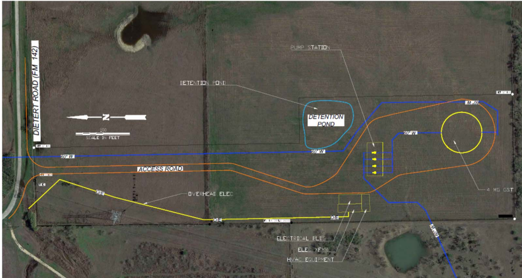
Figure 2-8 Intermediate Pump Station #2 Site Layout
