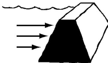
**Embankment dams** are good for damming broad streams. Heaping up earth, clay, and gravel and then pressing it down until it is packed and watertight make them. The top layer is close-fitting stone called riprap.
